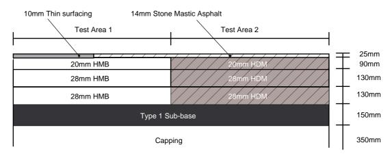
Figure 6 Construction thicknesses in M65 trial
