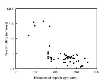
Figure C1 Rate of rutting versus thickness of asphalt layer
