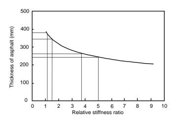
Figure E2 Relative stiffness ratio versus asphalt thickness
