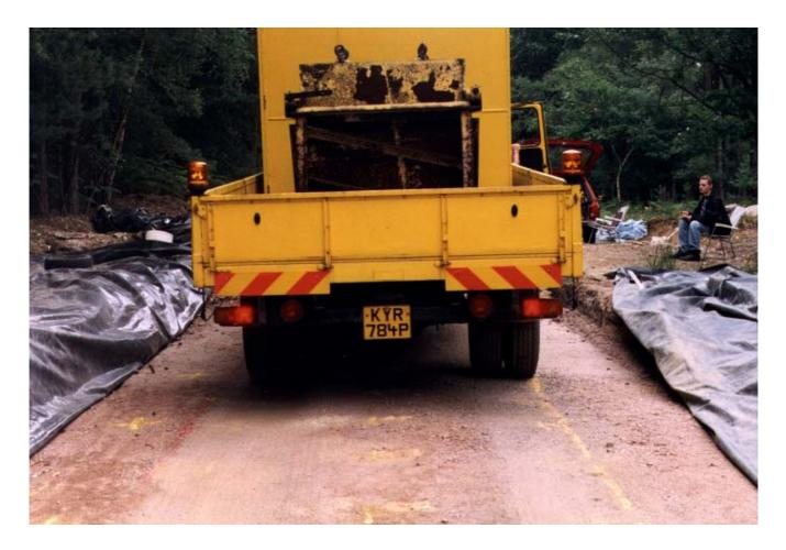
Figure B7 Lorry used for trafficking the trial foundations
