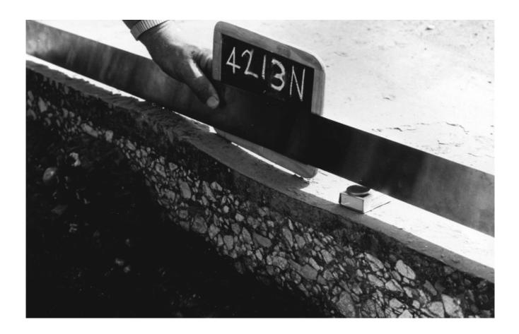
Figure A1 Surface rutting on a section of the M6
