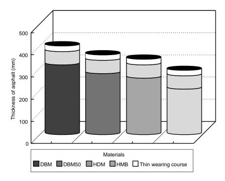
Figure 5 Pavement designs to resist surface rutting
