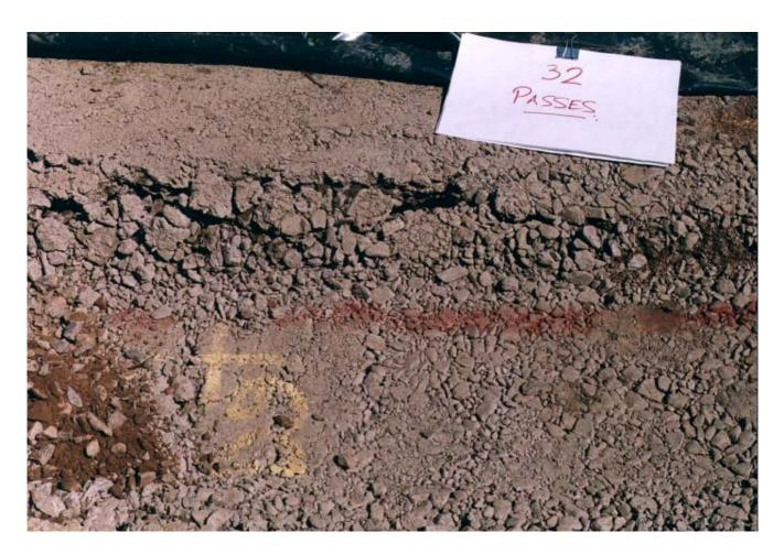
Figure B10 Failure of Section D after 32 passes
