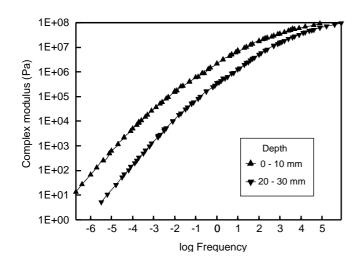
Figure A7 DSR master curves at 25°C illustrating increased binder ageing near surface
