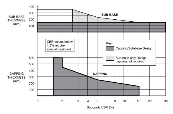
Figure 1 Capping and sub-base thickness design
