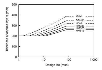
Figure E4 Design curve for high modulus roadbase (HMB)
