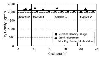
Figure B5 In-situ densities using NDG and sand replacement techniques
