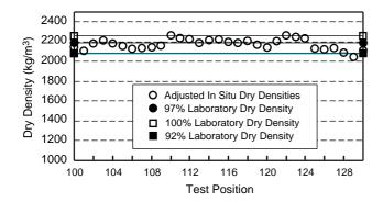
Figure B14 In-situ dry density on the completed foundation
