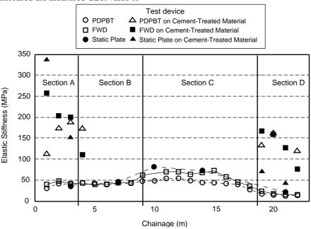
Figure B6 Measured stiffness values along the centre-line of the trial
