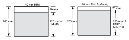
Figure 3 Illustration of roadbase adjustment using a thin surfacing
