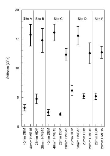
Figure E1 Mean ITSM and standard deviation of HMB15 and control materials
