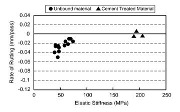
Figure B11 Rate of deformation under trafficking in comparison to foundation stiffness
