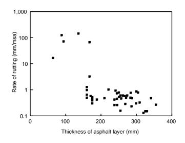
Figure A3 Measured rate of rutting of trunk roads with DBM roadbase
