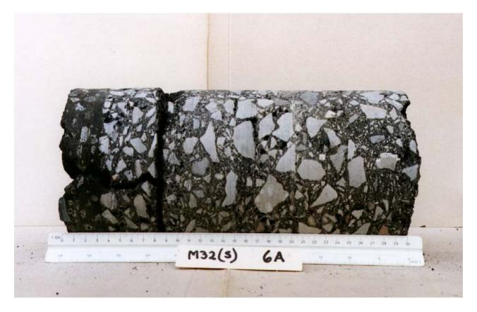
(b) Core showing depth of crack penetration
