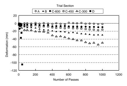
Figure B9 Cumulative foundation deformation under trafficking
