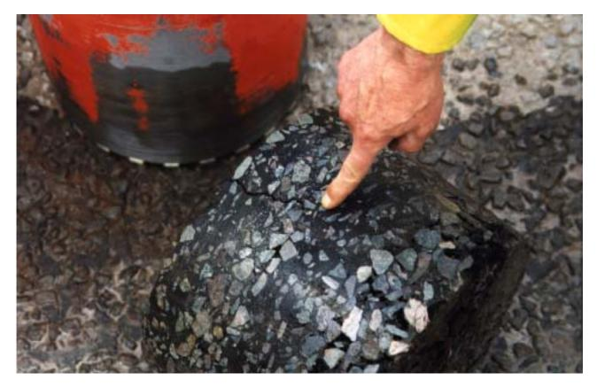
(b) Core showing depth of cracking penetration
