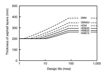
Figure 4 Design curve for high modulus roadbase (HMB)
