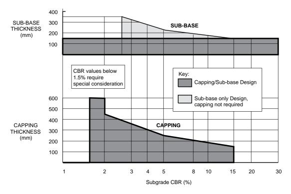
Figure B1 Capping and sub-base thickness design
