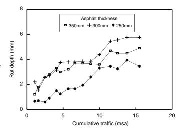
Figure A2 Rut development of experimental pavements
