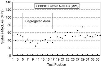
Figure B13 Stiffness at the formation (PDPBT results)
